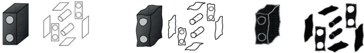
a) Default partition of nominal model b) Default partition of skin model (specification) c) Default partition of sampled surface model (verification)
