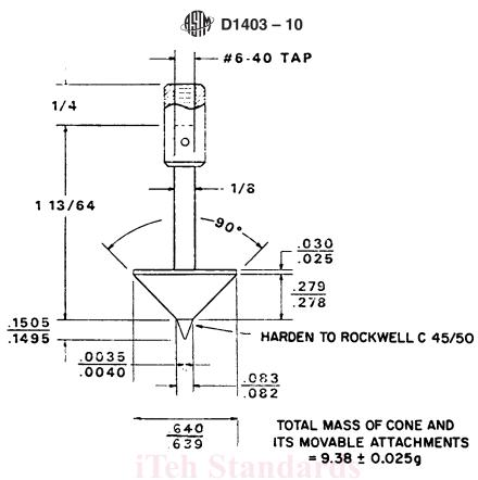
Note—All dimensions are in inches. Tolerance of fractional dimensions is  $\pm \frac{1}{64}$  in. ( $\pm 0.4$  mm).
