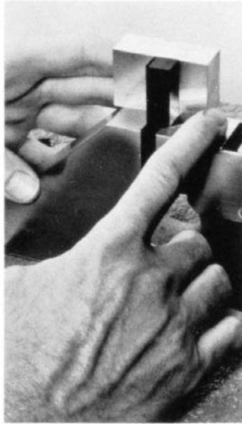
FIG. 4 Jig for Positioning Specimen for Clamping
