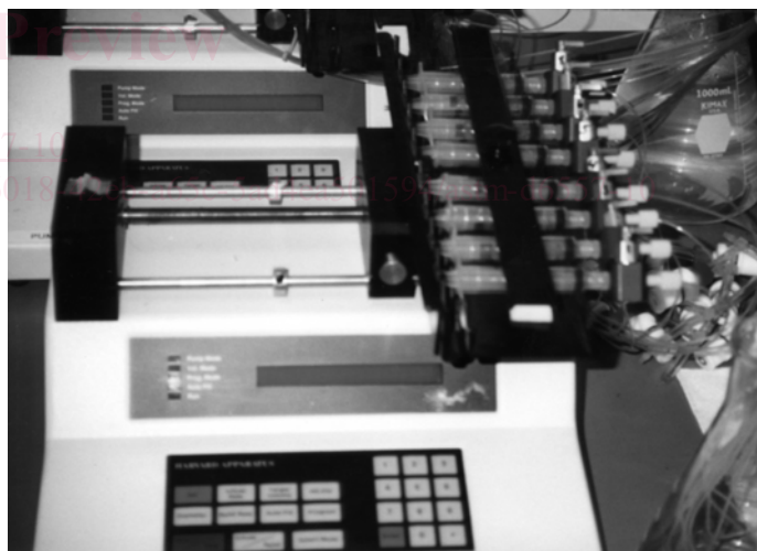
FIG. 3 Photograph of Acid Delivery System
