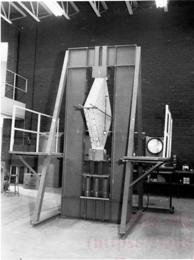
FIG. 1 Apparatus for Determination of Diagonal Tensile or Shear Strength Masonry Assemblages
