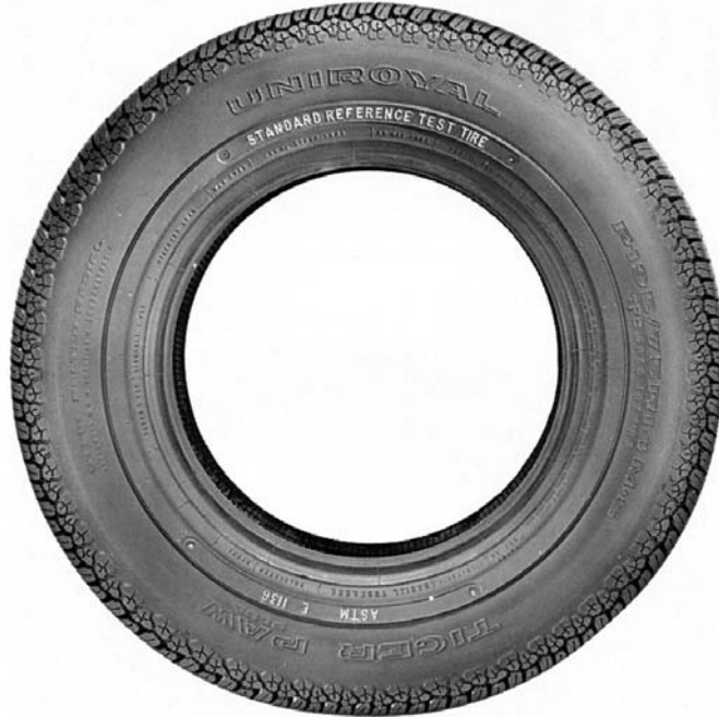
FIG. 2 Side View of a the P195/75R14 Radial Standard Reference Test Tire
