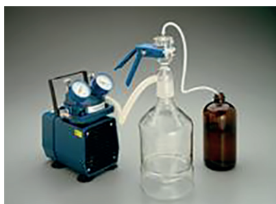
Figure 1 — Example vacuum filter set-up
