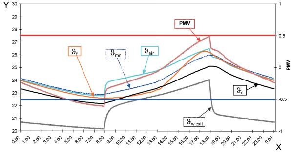
Kev Χ time, h Y temperature, °C **PMV** Predicted Mean Vote iTeh STANDARD PREVIEW  $\theta_{\rm air}$ air temperature (standards.iteh.ai) ceiling temperature  $\theta_{c}$  $\theta_{\mathrm{mr}}$ mean radiant temperature  $\theta_{\mathrm{f}}$ floor temperature ISO/DIS 11855-4 water return temperature/standards.iteh.ai/catalog/standards/sist/1046e7a4-5a49-41f5-89dc- $\theta_{\text{wexit}}$ 9ad76eedbe36/iso-dis-11855-4
