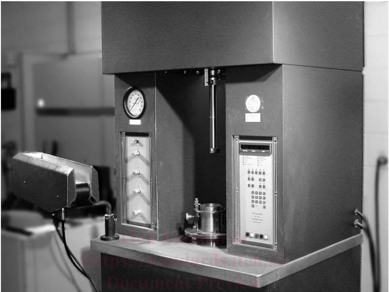
FIG. 2 Compactor with Sample Feed Trough
