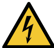
Figure 1 — Symbol of voltage class B electric components
