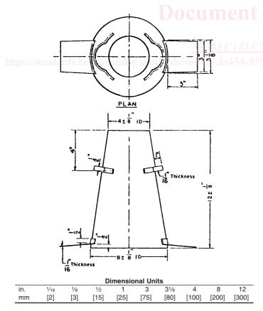
FIG. 1 Mold for Slump Test
