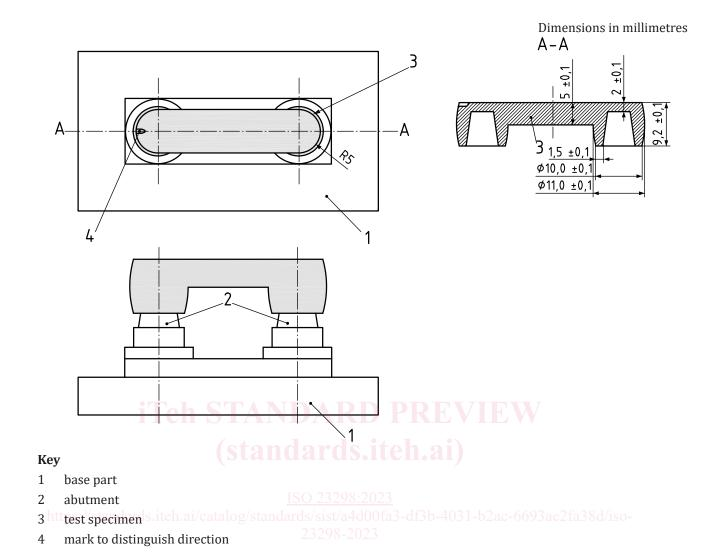
Figure 4 — Test specimen of the bridge
