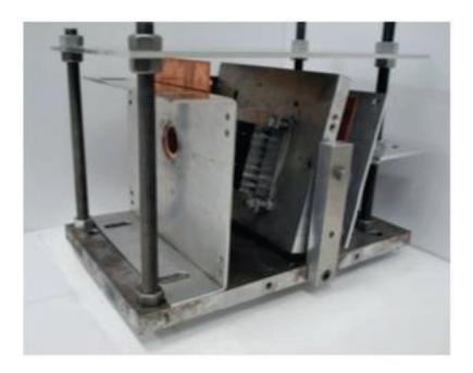
NOTE The front witness plate can be removed when the front ejecta is negligible.
