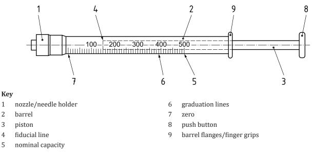
Figure 1 shows a manually operated precision laboratory syringe.
