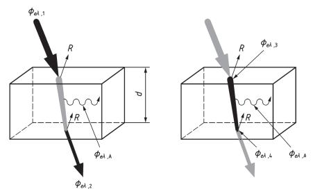
NOTE The light falls onto the surface at normal incidence, however, it is sketched at an angle in order to visualize the surface reflection *R*. That means, travel path of the light and geometrical thickness *d* are the same.
