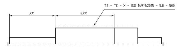
Figure 4 — Example for a thermally sprayed coating, top coat only, free choice of spray process, spray material in accordance with ISO 14919, areas coated (— - — - —), areas not allowed to be coated (without marking) and such areas which may be coated (- - - - -)
