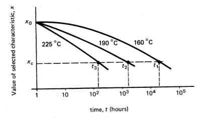
$x_{o}$  is the numerical value of the chosen characteristic at the beginning of the test;  $x_{c}$  is the critical (threshold) value of the same characteristic.
