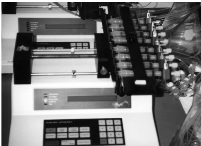
FIG. 3 Photograph of Acid Delivery System
