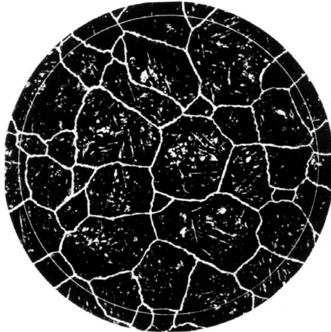
FIG. 4 Example of Austenite Grains in Steel from Plate IV. Grain Size No. 3 at 100X
