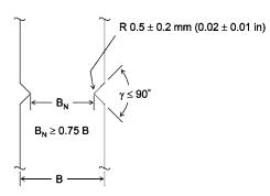
FIG. 6 Schematic of Side Groove Configration
