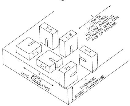
(a) Rectangular Sections—Specimens Aligned with Reference Directions
