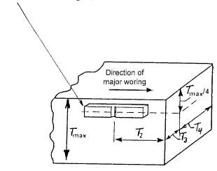
Note 1—For material with thickness T greater than 2 in. [50 mm],
