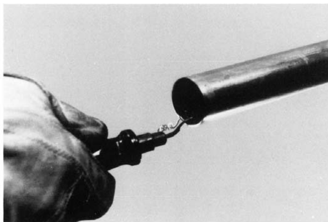
FIG. 5 Reaming: Deburring Tool
