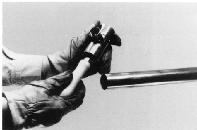
FIG. 9 Cleaning: Fitting Brush
