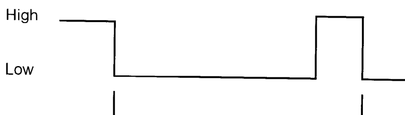
Figure 2: Start bit pulse format (standards.iteh.ai)
