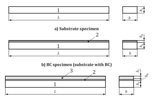
c) TBC specimen (substrate with both BC and TC)
