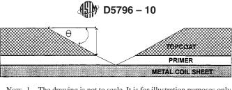
Note 1—The drawing is not to scale. It is for illustration purposes only. Note 2— $\theta = 5^{\circ} 42^{\circ} \underline{ft} 38^{\underline{n}} \underline{in}$ . Tan  $\theta = A/B = 0.1$ A = 0.1B FIG. 1 Typical Crater Formed by Boring Device
