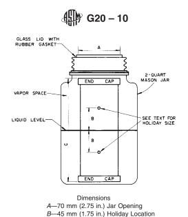
C-90 mm (7.00 in.) Length of Pipe Specimen
