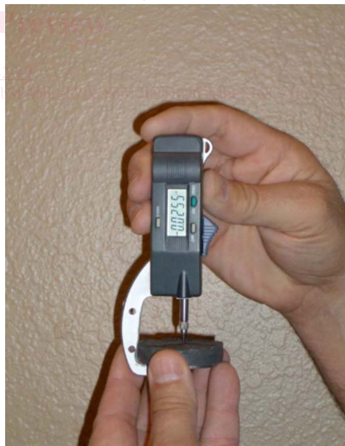
FIG. 2 Micrometer Measuring a Replica Coupon
