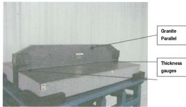
FIG. 4 Example of a Table and Granite Parallel Used to Measure Straightness by the Roll Test
