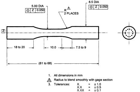
FIG. 1 Specimen Dimensions
