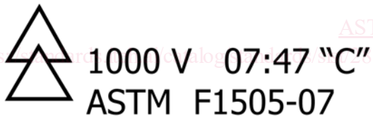
FIG. 6 Example for Insulation of the Handles of Tweezers (see 5.5)
