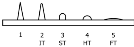
FIG. 1 Critical Temperature Points
