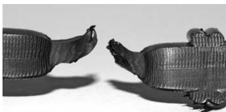
FIG. 2 Ductile Rupture Outside Fusion Interface
