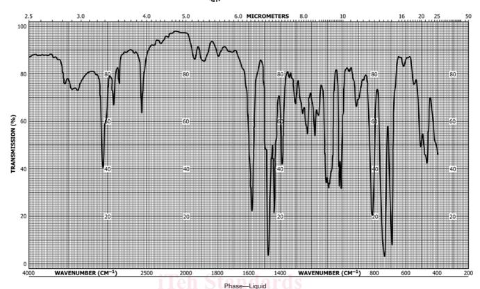
Prism-NaCl FIG. 1 Infrared Spectrum of Poly(phenylene sulfide) Pyrolyzate
