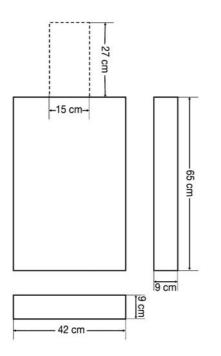
NOTE 1—The phantom container should be constructed so that the phantom material is of the dimensions shown in the figure. Dotted portion of the phantom is optional.
