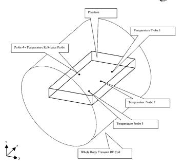
NOTE—Temperature probes 1, 2, and 3 are in the locations of greatest heating on or near the implant. Temperature probe 4 is the Temperature Reference Probe.
