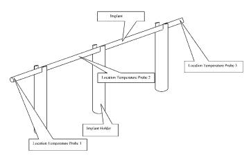
Note—Because implant holders with material differences from the phantom fluid will cause local field disturbances, temperature probes should be located at least 2 implant holder-diameters away from the implant holder to minimize the effect on the temperature measurements. For example, if an implant holder is 5 mm wide, the temperature probe should be placed at least 10 mm away from the implant holder.
