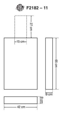
Note 1—The phantom container should be constructed so that the phantom material is of the dimensions shown in the figure. Dotted portion of the phantom is optional.
