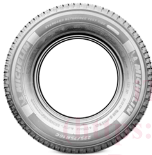
FIG. 2 Side View of the 225/75R16C 116/114S Radial Light Truck Standard Reference Test Tire
