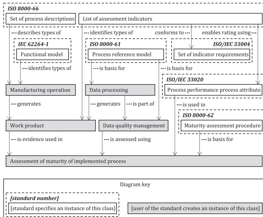
NOTE See ISO/IEC 19505-1 for details on the notation in this diagram.
