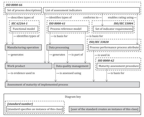
NOTE See ISO/IEC 19506-1 for details on the notation in this diagram.
