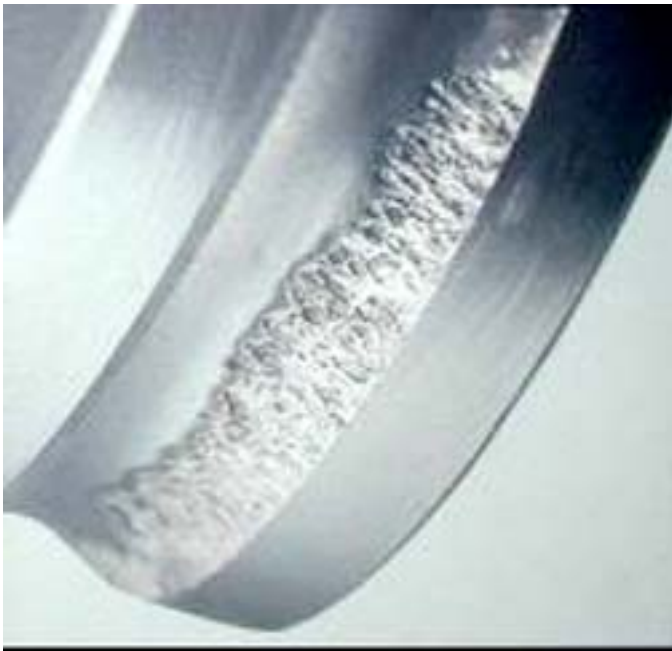
FIG. 2 Typical Bearing Spall
