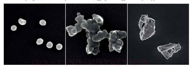
NOTE The images are projected views from certain angles of the 3D objects. Depending on the viewing angle, the observable size of particles can vary substantially.
