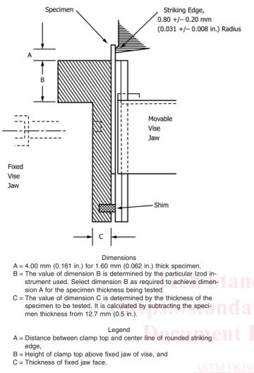
FIG. 1 Typical Specimen Clamping Device
