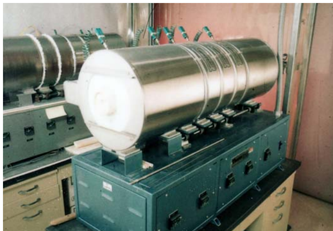
FIG. 3 Photograph of Typical Gradient Temperature Furnace
