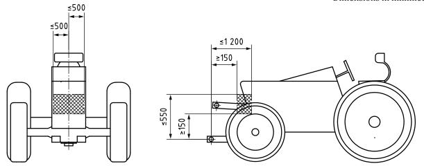
NOTE The dimensions based on lower hitch point are taken when the hitch point is horizontal with the draft arm pivot point.
