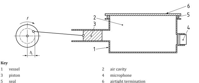
Figure 2 — Basic principle, termination with an airtight seal
