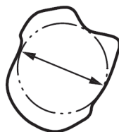
d) Section size obtained from a global linear size with maximum inscribed criterion (other criteria are possible)
