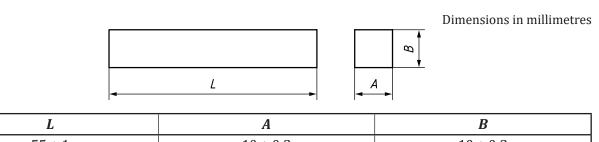
$55 \pm 1$   $10 \pm 0.2$   $10 \pm 0.2$  NOTE In order to have a robust tool design, a radius of up to 1 mm can be applied in the corners of the tool
