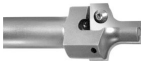
FIG. 1 Illustration of a Router Head With Insert Tooling
