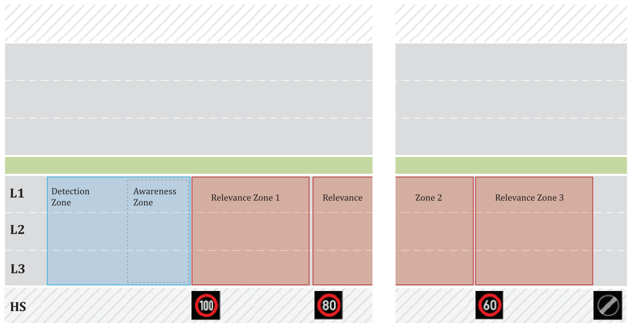
Figure 3 — Concatenated Relevance Zones (standards.iteh.ai)
