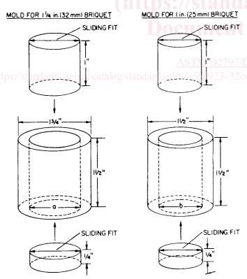
Note 1—Material: cold rolled or stainless steel. Dimensions a and b (inside diameters) are nominally 32 mm [1 $\frac{1}{4}$  in.] and 25 mm [1 in.]. If an automatic polishing attachment is to be used, these dimensions should be specified to yield a briquet fitting snugly in the briquet holder.
