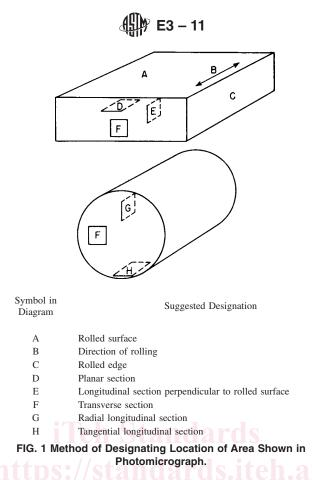
(0.5 to 1.0 in.) square, or approximately 12 to 25 mm in diameter if the material is cylindrical. The height of the specimen should be no greater than necessary for convenient handling during polishing.
